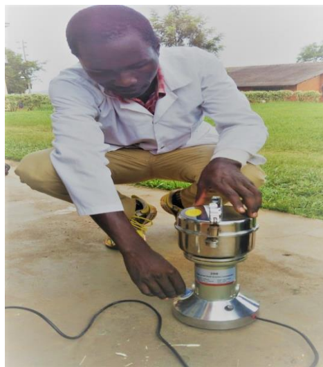
Figure 3: showing pretreatment process being done using high speed multi-function comminutor
